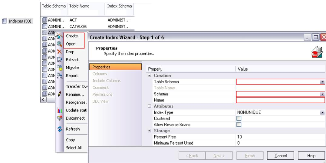
DBArtisan XE object properties correspond to CREATE *object\_type* and ALTER *object\_type* clauses, options, and keywords, appropriate to the object type and DBMS platform. In addition to basic properties, the wizards and editors offer object-specific options such as
