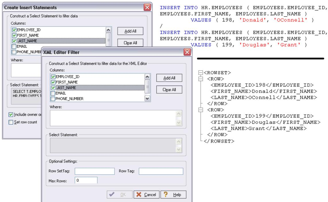
The **Extract Data As XML** feature provides a comparable function. It lets you make table data available in XML format. After qualifying records and columns, the resulting data is opened in an XML editor.
